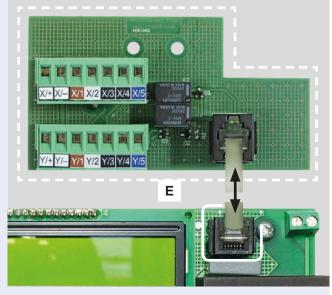
RJ-connection ST 64(A) with optional dropbolt module
