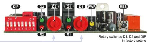
The Reset button (RES) has 2 functions which can be activated via the different duration of the key pressure:
