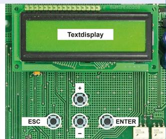
• AUTO-EXIT: If during programming no button is actuated for 1 minute or longer, the programming mode is left automatically. The control is set "ready" without storage of possibly changed values.
