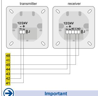
· Jumper J of transmitter and receiver has to be
