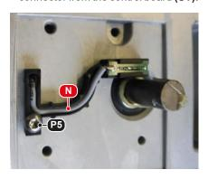
Guide the emergency release cable (N) of the emergency release motor through the rubber grommet in the opening (X) of the operator and plug it on the control board (ST) as shown.
