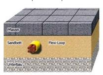
For laying under paving stones The Flexi-Loop is laid in the sand bed.
